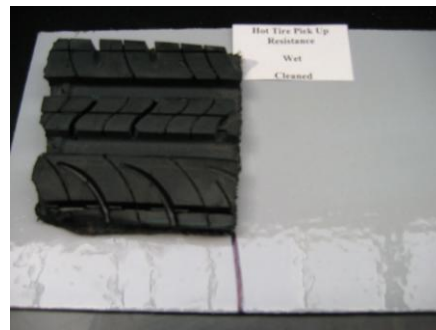
FIGURE 3. Wet Hot Tire Pick Up Resistance, Cleaned
